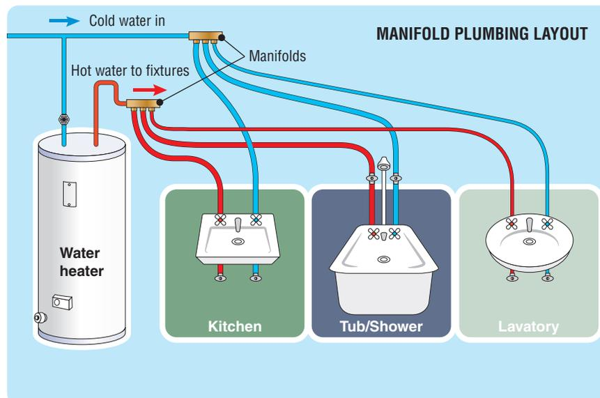
*A plumbing manifold system provides cutoff valves at the main terminus with flexible plumbing hoses that connect to the fixtures. Insulating the manifold and connecting lines is critical to reduce standby losses.*
