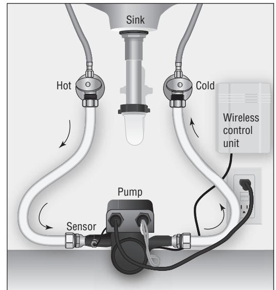
An on-demand hot water distribution system can be installed easily in new homes. As a retrofit solution, an on-demand pump can be installed at the furthest fixture from the water heater. A do-it-yourselfer can install such a unit under a lavatory sink. It involves shutting off the water main, adding hose "T" extensions to the cut-off valves and connecting bypass hoses to the pump (note: a GFCI electrical outlet is required to power the pump).
