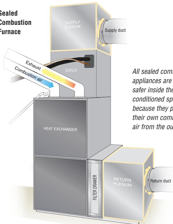
*All sealed combustion appliances are much safer inside the conditioned space because they provide their own combustion air from the outside.*
