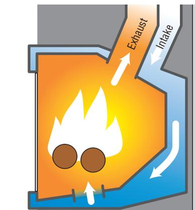
Gas log fireplaces should be a sealed combustion design because ventless gas fireplaces are unsafe.
