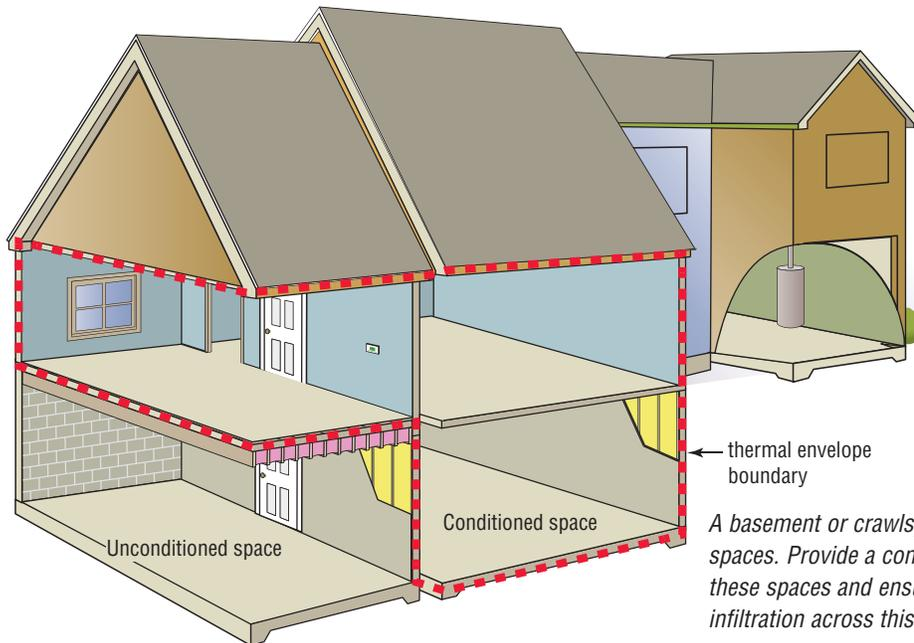
**Comfort, health and safety** are all improved when design principles and construction methods are based on proven building science and physics. This is achieved by looking at the whole house as a system to understand that performance is interconnected by its components.
